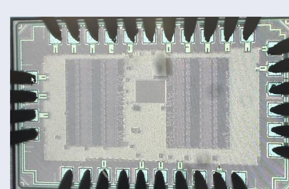
Chip microphotograph of a PUF macro comprised of a crossbar array of 16x16 PUF cells in 28nm CMOS technology
