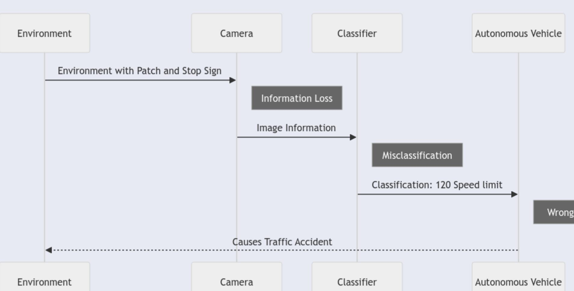
Sequence Diagram Illustrating the Step-by-Step Realization and Execution of an Evasion Attack Against the Perception and Decision-Making Systems of an Autonomous Vehicle
